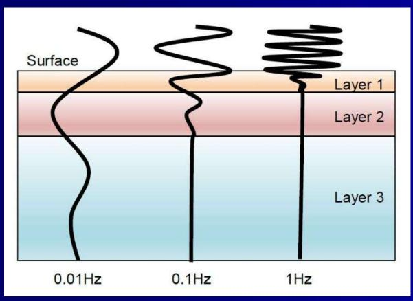
Electro-telluric currents are geo-magnetically induced currents that flow through conductive formations in the subsurface.
