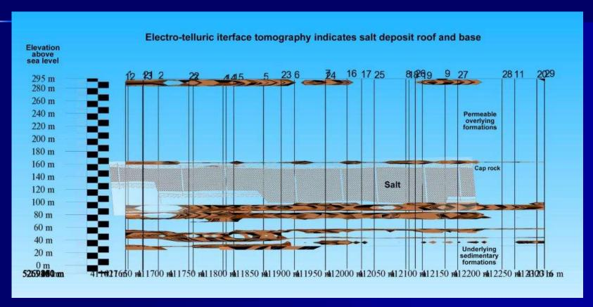
The salt layer has been determined with an accuracy of approx. +/- 1 meter.
